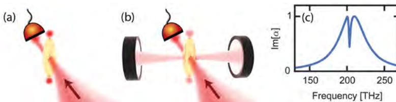
Figure 8.1: Cavity-induced modification of antenna polarizability (a) A single polarizable scatterer, probed in a transmission experiment. (b) A simple Fabry-Pérot cavity modifies the local density of states and alters the scattering properties of a plasmonic scatterer. (c) A spectrally narrow cavity mode can suppress the imaginary part of the polarizability \alpha of a plasmonic scatterer.
