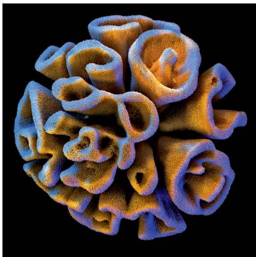
FIGURE S1: Self-assembled microarchitecture composed of \text{BaCO}_3 nanocrystals and amorphous \text{SiO}_2 (structure width: 26\ \mu\text{m} ).
