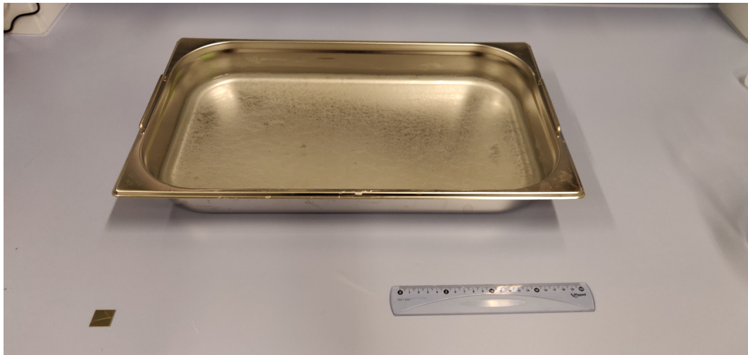
Figure 3.2: Scalability of DRB. Photo depicting yield difference between growth on the meniscus (tray) and on a substrate (aluminum slide, bottom left). Depicted ruler (bottom right) is 20 cm for reference.
