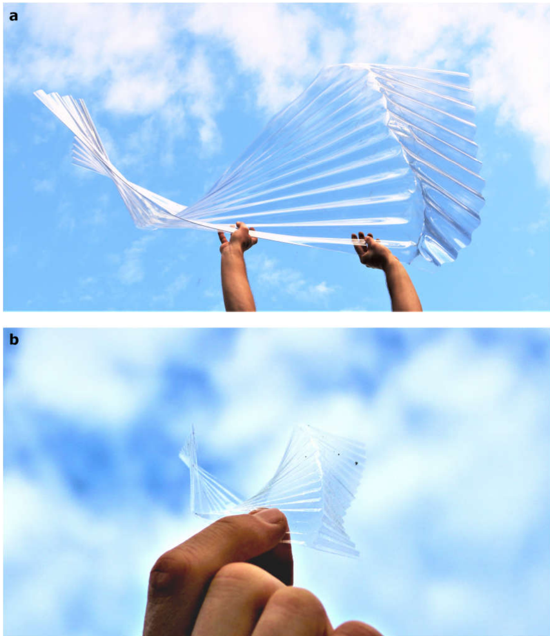
Fig. 5.7.: Groovy sheets of all sizes can reshape. a , A commercial plastic corrugated roofing sheet (1 mm thick, with groove wavelengths around 10 cm) is reshaped into a robust twisted configuration with the combined strength of two physicists. b , Plastic coating film, detached from corrugated craft paper. The film is 0.015 mm thick, with grooves around 0.5 cm. Although the two sheets differ by a factor of almost one hundred in size, they reshape the same way. Modelling courtesy of Hadrien Bense.
