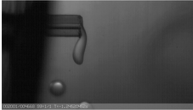
Figure 4.10 | Droplet formation at the capillary orifice at a rotation speed of 1000 rpm. Video recording of droplet formation at the capillary orifice at a rotation speed of 1000 rpm. The playback speed is 10 fps for a total of 250 frames. The capillary opening is 100 \mu\text{m} .
