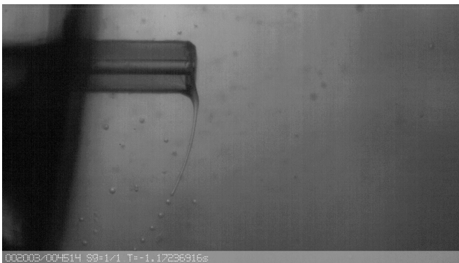
Figure 4.9 | Droplet formation at the capillary orifice at a rotation speed of 2700 rpm. Video recording of droplet formation at the capillary orifice at a rotation speed of 2700 rpm. The playback speed is 10 fps for a total of 250 frames. The capillary opening is 100 \mu\text{m} .
