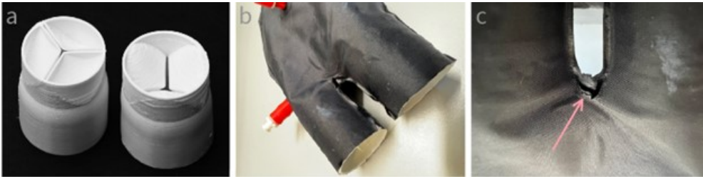
Figure A.9 | Fully soft prototype. a) Inlet and outlet valves 3D-printed from TPU. b) Placement of the valves in two separate openings. c) Rupture at the bottom of the U-shaped sealing line that separates the inlet and outlet valves.
