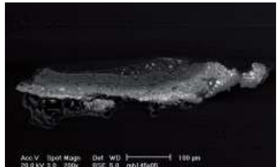
Fig. 17 Paint cross-section 145x05 from blanché and cupped paint lower right edge. Here the paint is built up in two layers of dark brown consisting mostly of organic brown earth pigment, possibly Cologne earth, in addition to a little red earth, on top of the lighter brown sketch layer. What appears to be a varnish layer separates the two brown layers. Normal light (A), UV (B) and SEM image (C)
