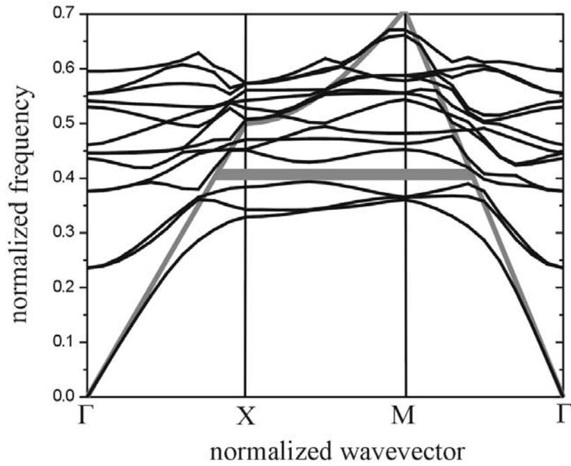
Calculated complete band structure for TM polarized light. Leaky and guided modes (solid black lines) are plotted above and under the light line (solid gray line), respectively. The guided modes exhibit a bandgap for normalized frequencies around 0.41 (gray bar).
