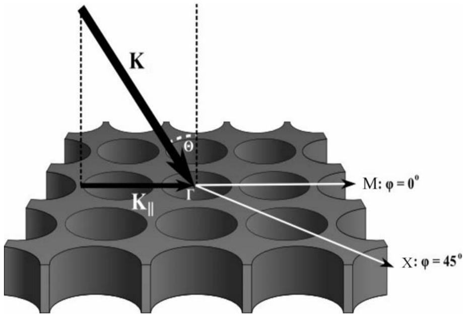
Schematic representation of the  $\mathbf{K}$  vector of the incident light projected on the plane of the slab. The in-plane wave vector of the incident light is  $\mathbf{K}_{\parallel}$  and is determined by the angle of incidence light  $\theta$ . The angle between the  $\Gamma$ - $X$  and  $\Gamma$ - $M$  crystal symmetry direction is  $45^\circ$ .
