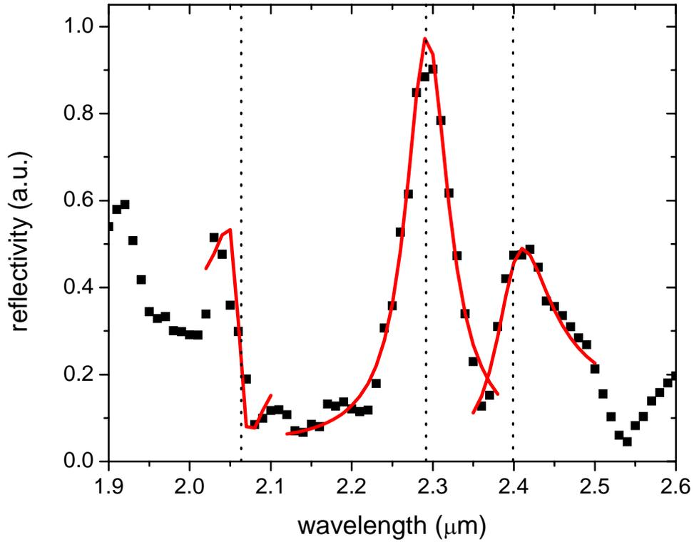
Example of a measured reflectivity spectrum with Fano-like line shapes. Squares: measured reflectivity for  $\Gamma$ -X symmetry direction, TM polarization, and  $10^\circ$  angle of incidence as a function of wavelength. Solid lines: Fano-line shapes fitted to three distinct reflectivity features. Dotted vertical lines: center wavelengths of the Fano line shapes.
