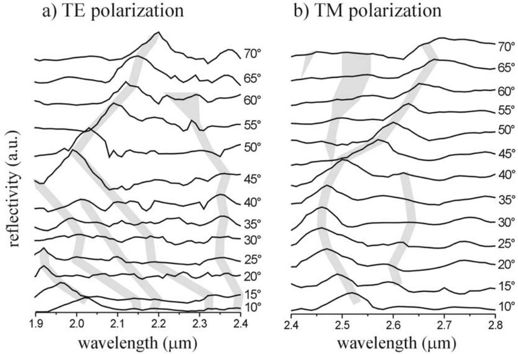
Reflectivity of the photonic crystal slab as a function of wavelength (black curves), measured along the  $\Gamma$ -M symmetry direction, a, for TE polarized and b, for TM polarized light. The curves are vertically shifted for clarity; from bottom to top, the angle of incidence increases from  $\theta = 10^\circ$  to  $70^\circ$ . The gray lines indicate reflectivity features.
