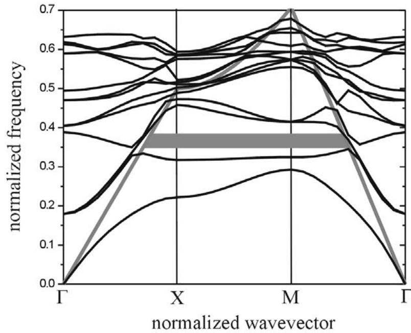
Calculated complete band structure for TE polarized light. Leaky and guided modes (solid black lines) are plotted above and under the light line (solid gray line), respectively. The guided modes exhibit a bandgap for normalized frequencies around 0.37 (gray bar).
