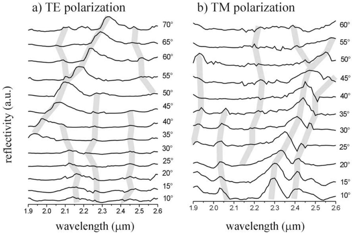
Reflectivity of the photonic crystal slab as a function of wavelength (black curves), measured along the  $\Gamma$ -X symmetry direction, a, for TE polarized and b, for TM polarized light. The curves are vertically shifted for clarity; from bottom to top, the angle of incidence increases from  $\theta = 10^\circ$  to  $70^\circ$  (a) and from  $10^\circ$  to  $60^\circ$  (b). The gray lines indicate reflectivity features.
