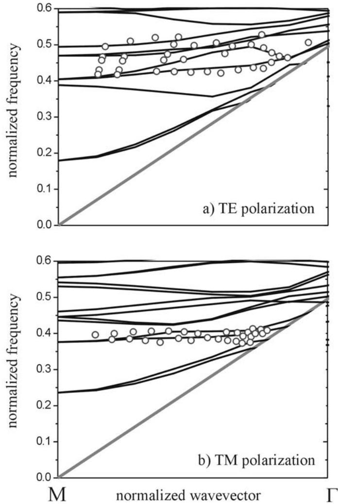
Out-of-plane band structure for  $\Gamma$ -M symmetry direction, a, for TE polarized light and b, for TM polarized light. The graphs show the dispersion obtained from the reflectivity experiments (open circles) together with calculated dispersion curves of the leaky modes (solid lines) above the light line, i.e. the dispersion of light in air (gray line).
