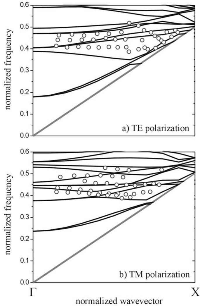
Out-of-plane band structure for  $\Gamma$ -X symmetry direction, a, for TE polarized light and b, for TM polarized light. The graphs show the dispersion obtained from the reflectivity experiments (open circles) together with calculated dispersion curves of the leaky modes (solid lines) above the light line, i.e. the dispersion of light in air (gray line).
