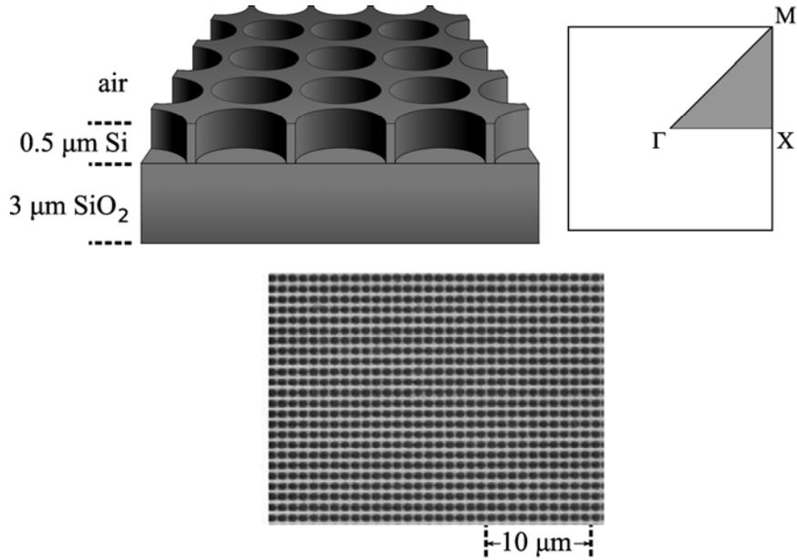
Upper left: schematic of the 2D photonic crystal consisting of a square lattice of holes in silicon. Upper right: Corresponding irreducible Brillouin zone with the high-symmetry points  $\Gamma$ , X and M. Lower: SEM micrograph of the photonic crystal, top view.
