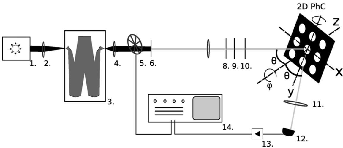
Experimental setup for specular reflectivity measurements. The individual components are: 1, QTH light source; 2, lens; 3, monochromator; 4, lens; 5, optical chopper; 6, slit; 7, lens; 8, pinhole; 9, low-pass filter; 10, polarizer; 11, lens; 12, detector; 13, amplifier; 14, lock-in amplifier.
