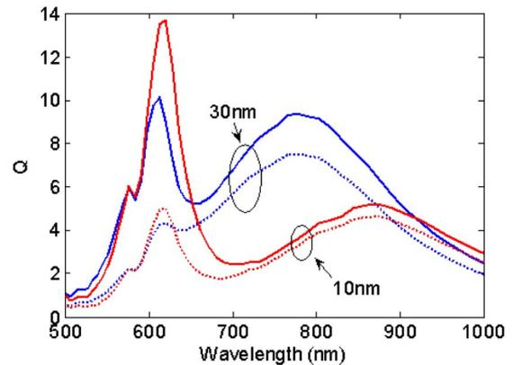
FIG. 4. (Color online) The total scattering cross section (solid lines) and scattering cross section of light scattered into the substrate (dashed lines), both normalized to geometrical cross section, for Ag cylinders on  $\text{Si}_3\text{N}_4$  underlayers on Si with thicknesses of 10 nm (red lines) and 30 nm (blue lines). The cylinders have a diameter and height of 100 nm and have a 30 nm  $\text{Si}_3\text{N}_4$  overcoating.
