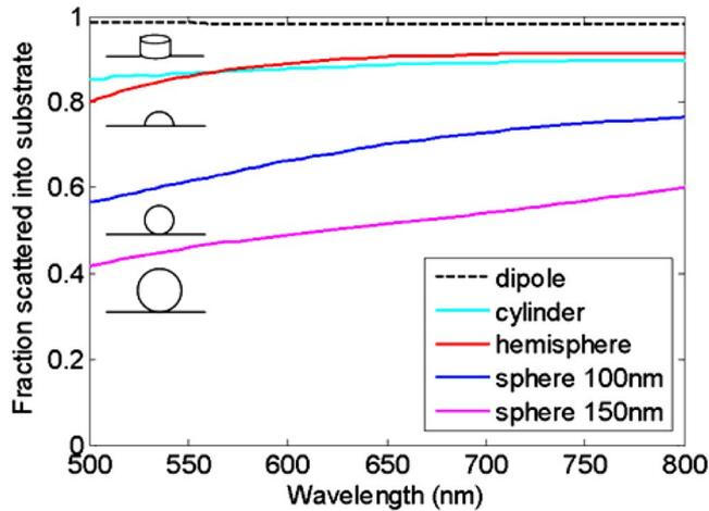
FIG. 1. (Color online) Fraction of light scattered into the substrate,  $f_{\text{subs}}$ , for Ag particles on a 10 nm thick  $\text{SiO}_2$  underlayer on Si: a cylinder with diameter  $d=100$  nm and height  $h=50$  nm; a 100 nm diameter hemisphere; a 100 nm diameter sphere; and a 150 nm diameter sphere. Also plotted is  $f_{\text{subs}}$  for a parallel electric dipole that is 10 nm from a Si substrate.
