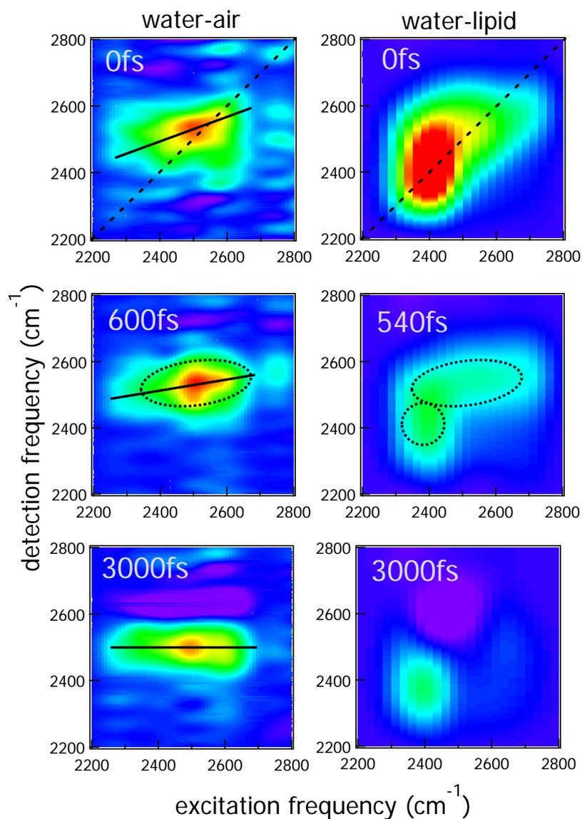
**Figure 2.** 2-dimensional SFG spectra of the D2O water-air (left column) and water lipid (right column) interfaces at various pump-probe delay times indicated in the graphs. The dashed lines in the upper panels denote the diagonal; the solid lines in the left column indicate the average slope of the diagonal peaks. Dotted circles/ovals indicate different water types.
