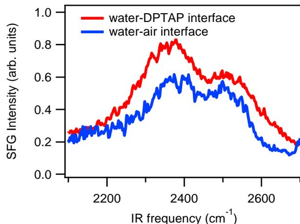
Figure 1. Normalized SFG spectra at the D<sub>2</sub>O water-air (blue) and water-lipid (DPTAP, red) interfaces. Note the remarkable similarity. The spectrum for the water-lipid interface has been offset by 0.2 for clarity.
