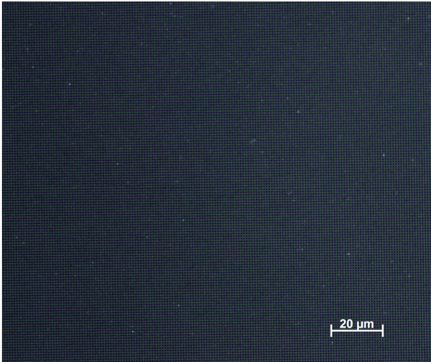
Figure 4.5: Dark-field optical microscope image of Ag nanowire network. The pitch of the array is 1000 nm.
